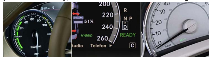
Fig. 4. Ready state indication on: Audi A8 hybrid , Mercedes S400, Chrysler Aspen Hybrid
