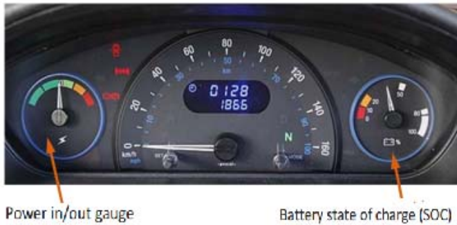
Fig. 1. Example of analog gauges dashboard with SoC and Power in/out gauge
