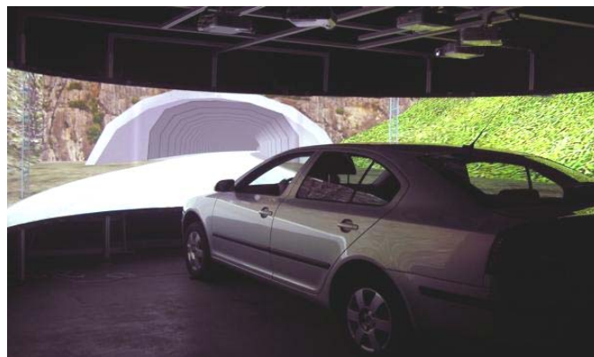
Fig. 8 driving simulator Octavia II developed by FD CTU in Prague [12]
