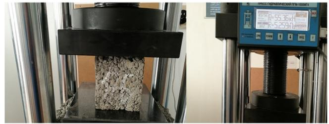
Fig. 3. Determination of the strength of the samples.
