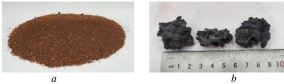
**Fig. 1** Ferrous sand (a) and iron ore agglomerate (b)
